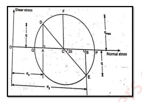
$\sigma_{N2}$  = Minor principle stress = L(OQ) \* Scale = 1\*10 = 40 N/mm<sup>2</sup>
