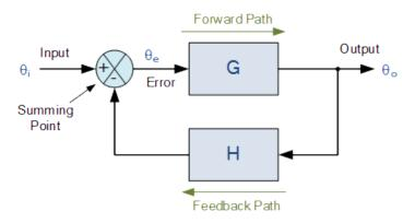
A closed loop system is also referred as a feedback control system. These systems record the output instead of input and modify it according to the need. It generates preferred condition of the output as compared to the original one. It doesn't encounter any external or internal disturbances.
