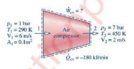
Apply the steady state energy balance between (1) and (2) gives
