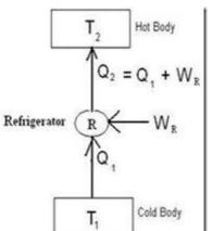
3. A heat pump is similar to a refrigerator. The only point of difference between the two is of the operating temperatures. The working temperatures in a refrigerator are of the colder level and atmosphere, whereas working temperatures in heat pump are of hotter level and
