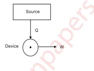
A PMMSK is a hypothetical device which working cyclically, receives energy as heat from a single thermal reservoir, and delivers as equivalent amount of work. The Kelvin-Planck statement of the second law tells us that it is impossible to constructs a perpetual motion machine of the second kind.
