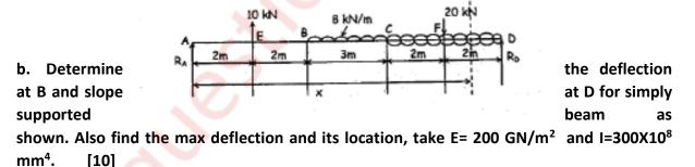
$EI = 200 \times 10^3 \times 300 \times 10^8 = 6 \times 10^{15} \text{ Nmm}^2 = 6 \times 10^6 \text{ KNm}^2$
