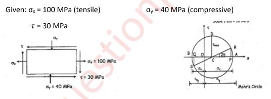
Step 1: Select scale 1 cm = 10 MPa. Select origin O, take  $\sigma_x = 10 \text{ cm}$  as OP and  $\sigma_y = 4 \text{ cm}$  as OD.
