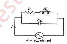
Consider a parallel circuit consisting of a coil and a capacitor as shown below. The impedances of two branches are:-
