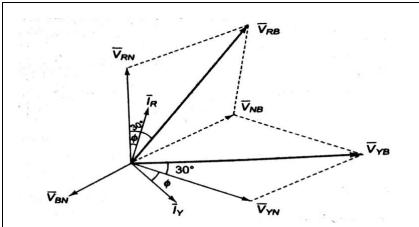
From phasor diagram, it is clear that phase angle between  $V_{YB}$  and  $I_Y$  is (30° +  $\varphi$ )
