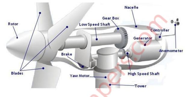
The schematic of the wind turbine components are shown here.
