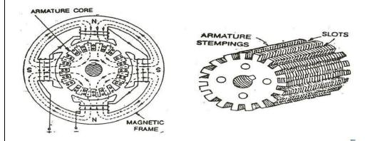
The armature core of a DC generator or machine serves the following purposes.
