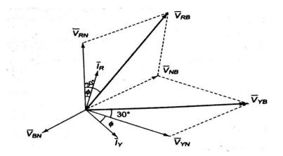
From phasor diagram, it is clear that phase angle between  $V_{YB}$  and  $I_Y$  is  $(30^\circ + \varphi)$
