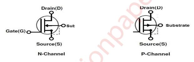
ii) The symbols for depletion mode of MOSFETs in both N-channel and P-channel types are shown above. In the above symbols we can observe that the fourth terminal substrate is connected to the ground, but in discrete MOSFETs it is connected to source terminal.
