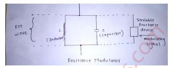
iii)The net result is to change the resonant frequency of the LC circuit by amounts proportional to the instantaneous a.f. voltages applied to the grid of the modulator tube, without changing the resistance of the LC circuit or the amplitude of the oscillations.
