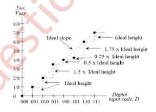
With respect to DAC define the term DNL. Determine the DNL for 3-bit non-ideal DAC whose transfer curve is as shown in figure. Take  $V_{REF}$ = 5V.
