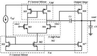
Design the given 2 stage operational amplifier for the given specifications.
