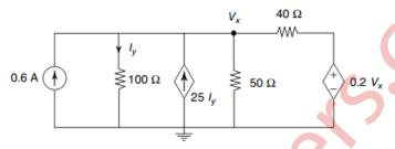
Q4 a Find the voltage V using superposition theorem.
