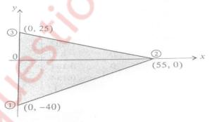
Nodal displacements are given as  $U_1 = 2$  mm,  $U_2 = 0.4$ mm,  $U_3 = 3$  mm,  $V_1 = 1$  mm,  $V_2 = 0$  mm &  $V_3 = 1$  mm. Find the stiffness matrix equation.
