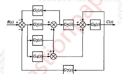
B) Find overall transfer function C(s)/R(s) for the given signal-flow graph using mason's **10 Marks** gain formula.
