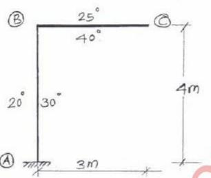
(b) Develop the stiffness matrix for prismatic member AB with reference to the 06 co-ordinates as shown in fig.
