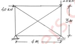
Work out the vertical deflection of point C due to change in temperature as indicated. Take thickness of each member 400 mm. and  $\alpha_t$  =12x10<sup>-6</sup>/° C E=200 GPa
