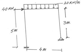
4. (a) Determine forces in each member of pin jointed frame as shown. Use force method. A=200 mm<sup>2</sup>, E=200GPa.
