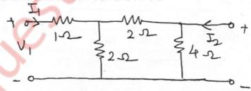
Q.2 (a) In the given network; what will be the value of  $R_L$  to get max. power delivered to it. (10)
