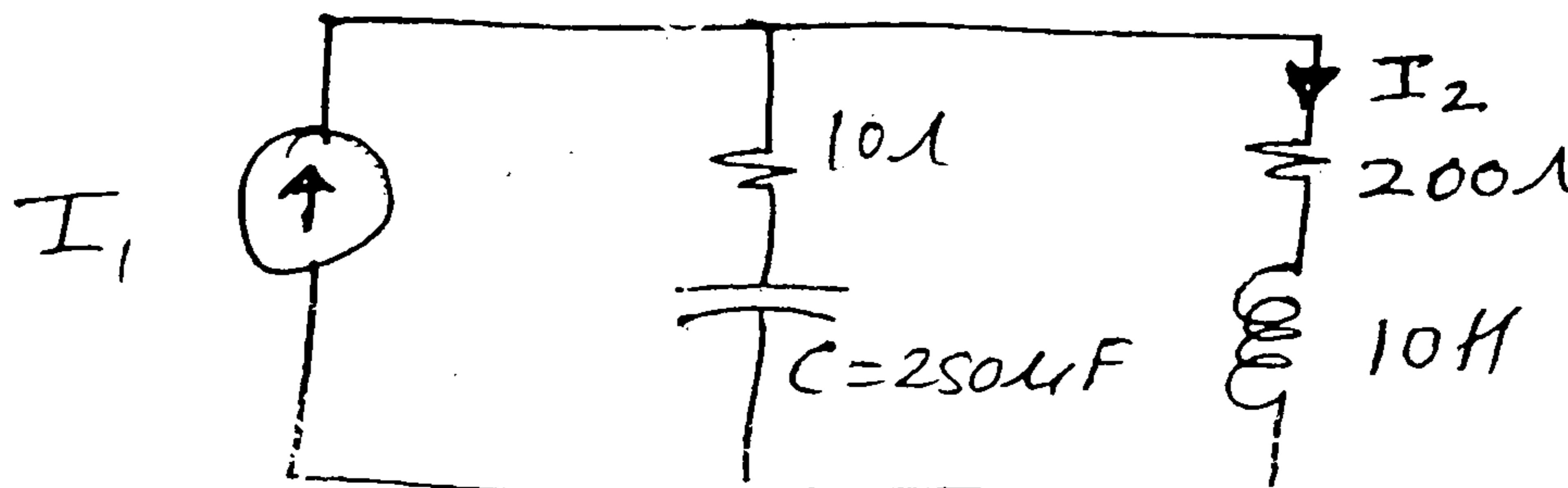
6. (a) For the Network shown below determine  $R_L$  for maximum power transfer and also determine  $P_L$
