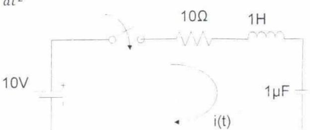
Q3 b) In the network shown, the switch is initially at position 1. On the steady state having reached, the switch is changed to the position 2. Find current i(t).
