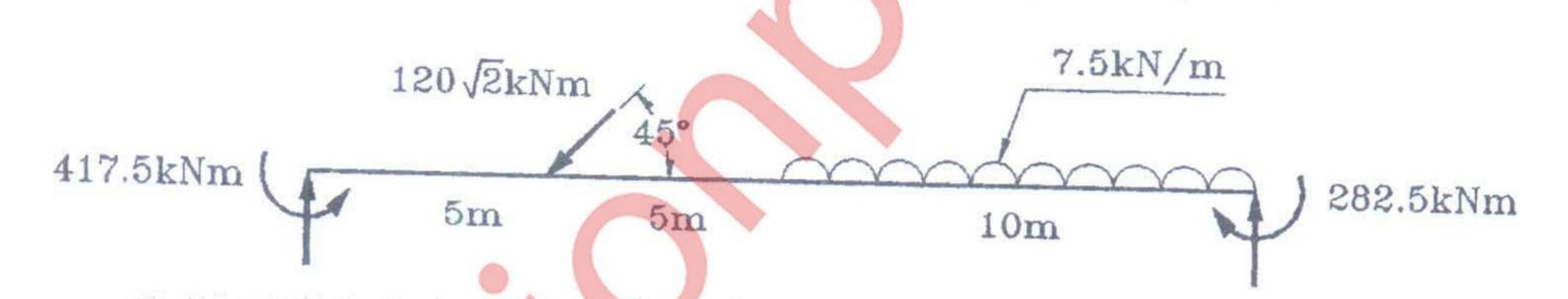
b. Determine the slope and deflection at the free end of the beam loaded as shown in the figure. E=200 GPa,  $I=14\times10^{-6} \text{ m}^4$
