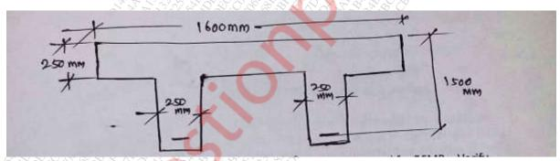
Total area of prestressing steel is  $4700 \text{mm}^2$ ,  $f_p=1600 \text{MPa}$  and  $f_{ck}=56 \text{MPa}$ . Verify its safety in limit state of strength flexure if ultimate moment acting at the section is 5000 kN-m (inclusive of self weight).
